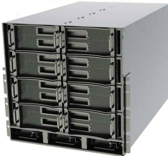
Figure 5. An SGI UV 3000 chassis enclosure (up to 4 per rack)
