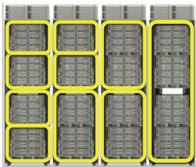
Figure 3. Examples of partitioning SGI UV 3000.
