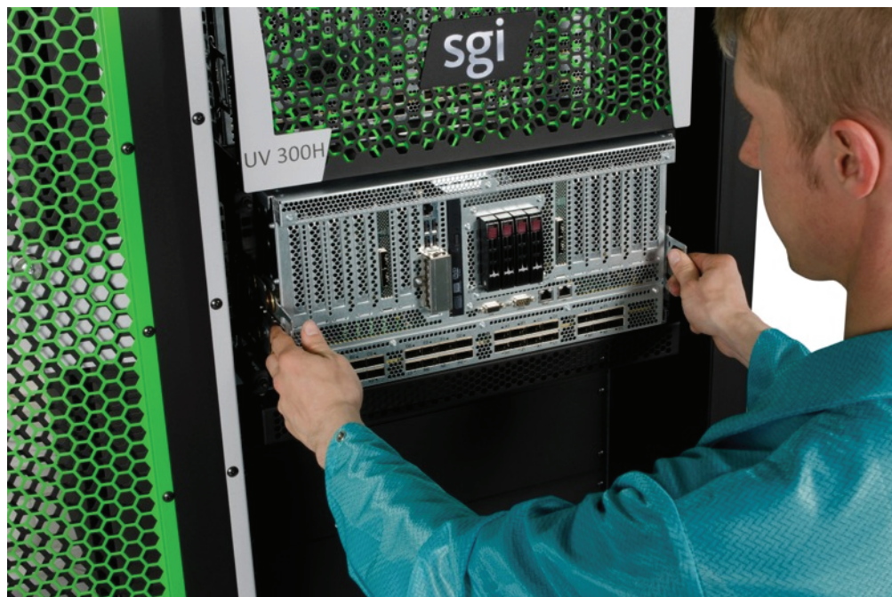
Figure 5. An SGI UV 300 chassis enclosure (up to 8 per rack)
