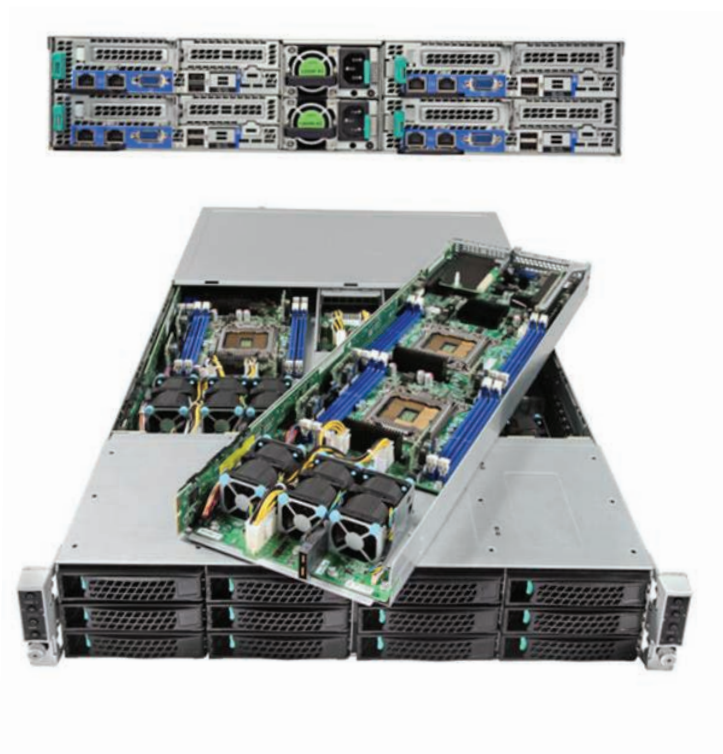
Figure 1: Overhead View of SGI Rackable Server with the Top Cover Removed
