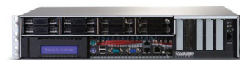
Application Node: SGI Rackable C2005- RP1 server with Intel Xeon Processor E5 Family
