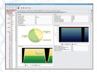
The Power Tab of SGI Management Center allows a system administrator to monitor per node, per rack and per system power usage, in both kW and in cost, depending upon the cost/kW factor entered into the tool. Active policies that are in place can also be viewed quickly from this display.
