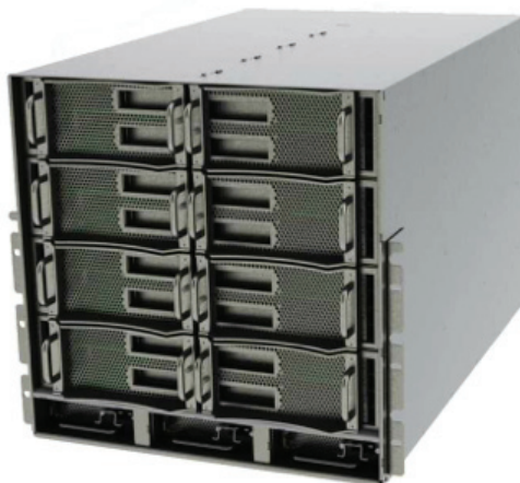
Figure 3. An SGI UV 2000 enclosure (four per rack) supports up to 8 UV 2000 compute blades.
