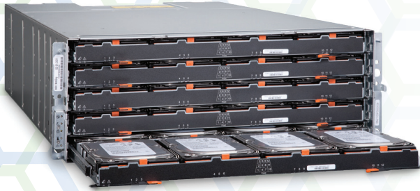
Front of the IS5500-60: 60 3.5-in or 2.5-in drive enclosure
