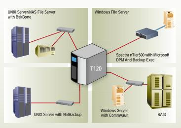
With support for multiple connectivity protocols as well as all major backup software packages and operating systems, the T120 system fits easily into any environment. With Shared Library Services (SLS) the T120 can easily be configured to use partitions and simultaneously support multiple generations of LTO technology and different connectivity protocols.
