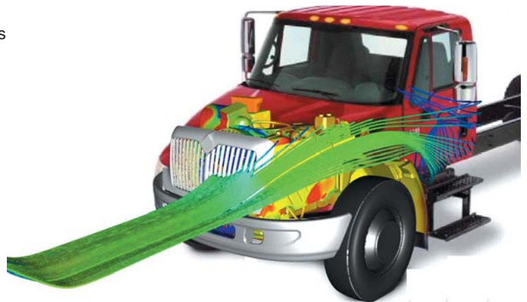
Figure 1: CFD Analysis of Full Vehicle Air Flow of a Class 5 Truck
