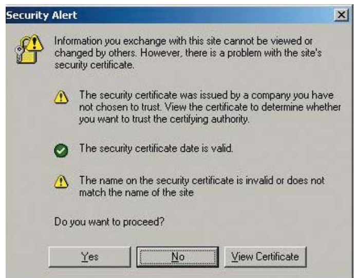
Figure 1. All the features of SGI InfiniteStorage Resource Manager are delivered through a Web browser and a secure HTTPS connection controlled by username and password authentication pairs. In compliance with the Storage Management Initiative Specification [SMI-S], SGI software asks users authenticating via HTTPS about accepting keys from non-recognized authorities.
