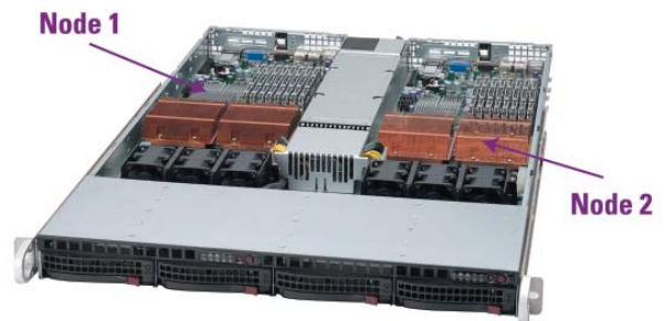
Figure 1. SGI Altix XE310: Two Nodes on a Single Board
