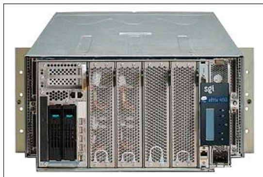
SGI RASC Appliance for Bioinformatics 8.25" high chassis for standard 19"
