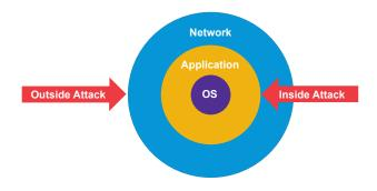
For **network security**, industry standards have been developed for firewalls, virtual private networks, and network encryption in order to ensure data integrity and to prevent network intrusion, denial of access, data theft, and other attacks. Networking hardware and software and network security have become a standard part of a computer system.
