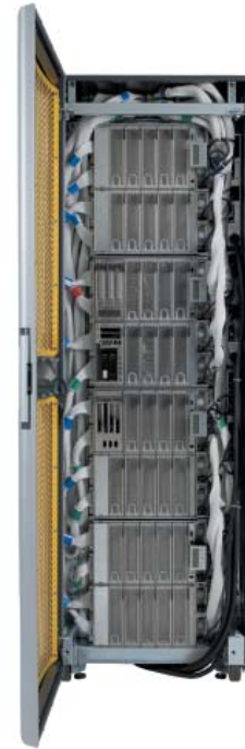
Figure 3. Altix 4700 tall rack containing 4 IRUs
