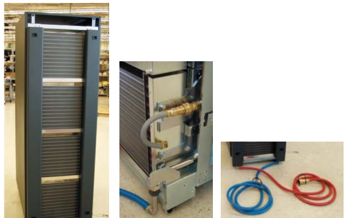
Figure 1. Details of SGI water cooling available for Altix 4700 server deployments.
