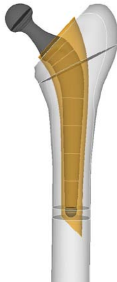
Patient Specific Positioning – replicating the placement of the hip implant in a 3D solid model representing the patient's anatomy [dark gray = implant, gold/brown = cement mantle, light gray = femur]
