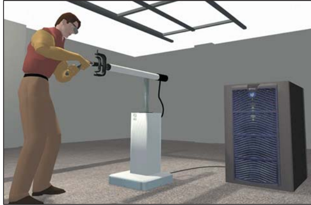
The Virtual Reality Trainer uses a real welding torch attached to a device that simulates pressure and resistance, a head-mounted display to view the 3D computer-generated environment, and a tracking system for both the torch and the trainee's head to monitor and display all movements in the virtual workspace.
