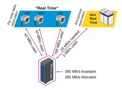
As soon as SD2 becomes active (T+1), and 42MB/s are needed for this station, GRIO will throttle down the (non priority) file recorder station to the remaining available bandwidth (from 25MB/s to 2 MB/s) and then will allocate 42MB/s to SD2.
