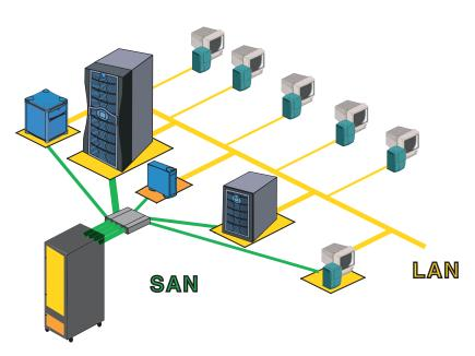
In the SAN with CXFS Shared Filesyetem example, each computer uses the same large CXFS shared filesystem (in yellow). There is no need to transfer data from one computer to another using the Ethernet network because data resides on the same equally accessible filesystem. This simplifies the data workflow and optimizes the available disk space by removing the need to duplicate files.
