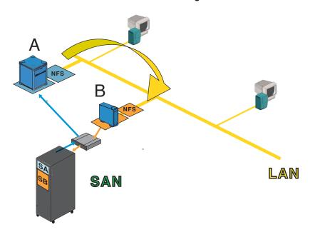
Because computers cannot natively share the same SAN array, data must flow from one part of the storage array (SA, owned by A) to another part of the same storage array (SB, owned by B) through the network. This transfer of data wastes disk space, network resources, and user time.
