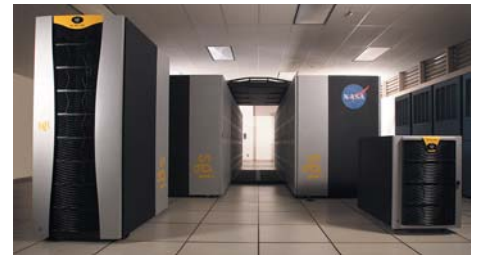
Recently, NASA Earth sciences researchers doubled the size of the agency's SGI Altix™ system - achieving 512 processors in a single image, by far the largest supercomputer ever to run on the Linux® operating system.
