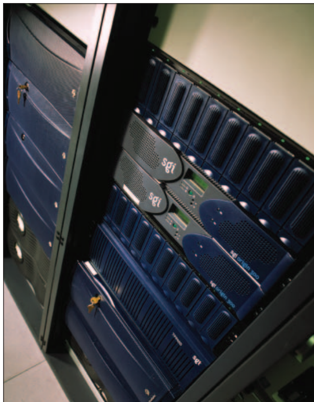
SGI Media Server for broadcast systems along with SGI Origin 300 servers provide ingest, storage, editing and playout functionality for SWR's new digital infrastructure.
