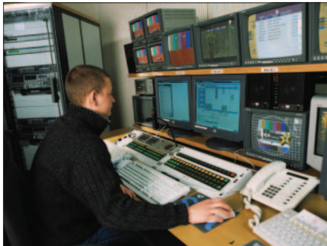
The SGI infrastructure allows operators to schedule, insert, edit and play out all over a gigabit ethernet backbone.
