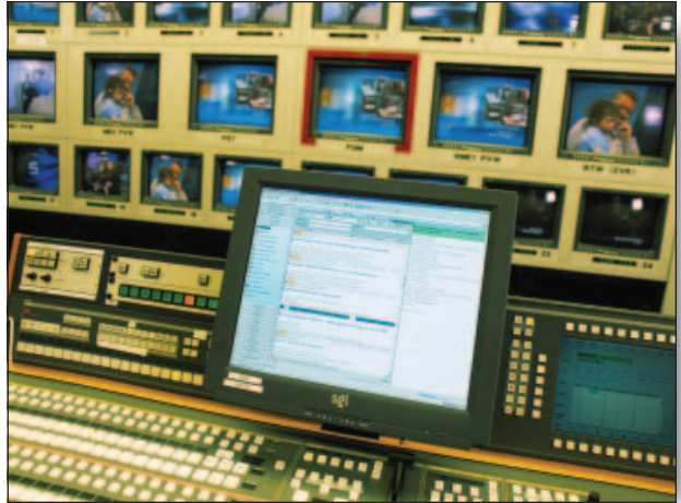
Faster time-to-air is achieved with the seamless integration between newsroom and automation software in the new SWR tapeless system.
