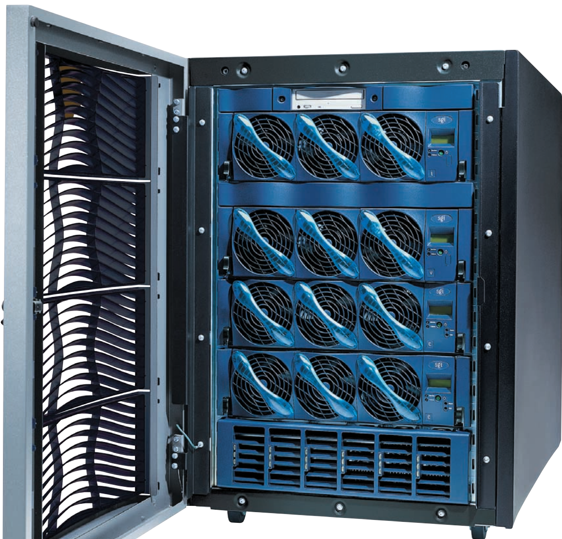
The 'entry level' Altix 3300 server is a half rack device which can accommodate up to 12 Itanium 2 processors and 96GB of pooled memory.
