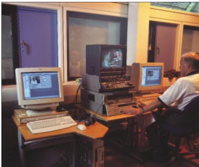
Danish Broadcasting operator shown here performing ingest using Keyvia's (formerly Keops) Key-MediaWorks – creating and checking in multi-resolution assets to the asset management system from VTRs and satellite.
