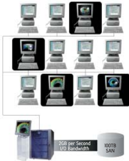
Fig. 1. An SGI Onyx 350 system with InfinitePerformance graphics supporting four virtual power users at a time in a departmental setting
