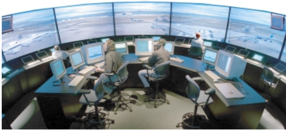
NASA's new FutureFlight Central facility is a full-scale air traffic control tower that tests ways to solve potential air and runway traffic problems at commercial airports.
