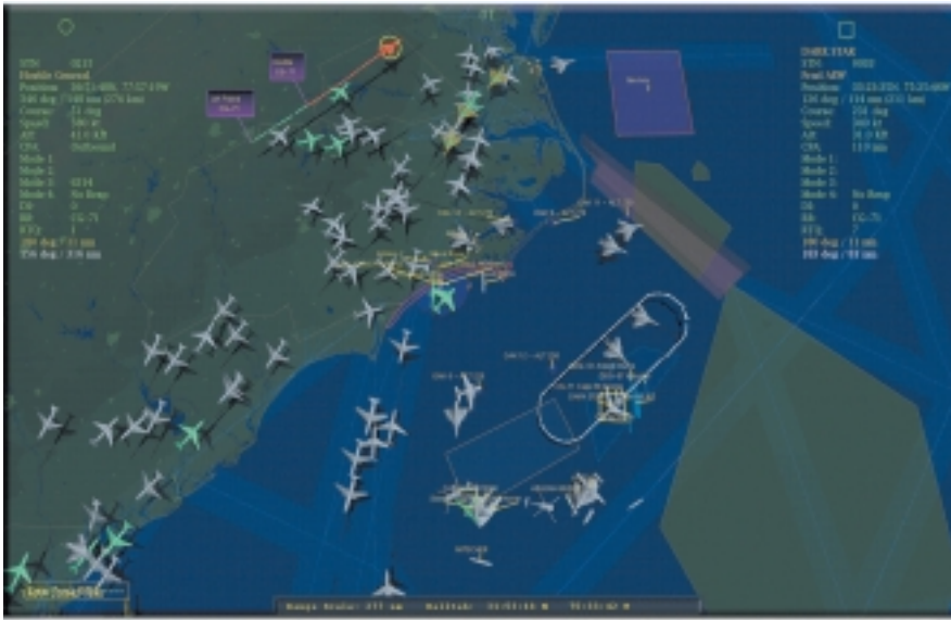
All known hostile and friendly aircraft are represented on the commander's screen in the AADC. Friendly units are shown in white, with silhouettes exactly matching the type of aircraft. Hostile units appear in red, commercial aircraft are green and unidentified craft are yellow.
