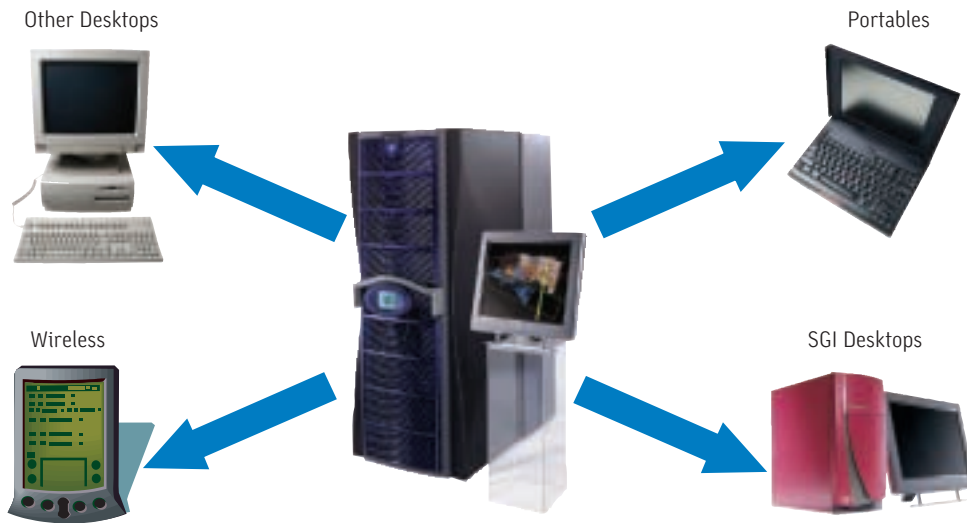
Fig. 2. Grid users can access the advanced visualization abilities of SGI Onyx family systems from anywhere on the grid using OpenGL Vizserver. A single Onyx family system can serve the visualization needs of several grid users simultaneously. Collaborative sessions can be established in which multiple users can see and manipulate the same visualization.
