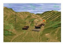
TOPSCENE 400, which offers midrange performance at significantly reduced cost, runs on the Silicon Graphics® Octane® desktop workstation. The Model 400 uses the same database as the Model 4000, but its hardware economics make it far more deployable. Its simulations are much like those generated by the Model 4000, but at reduced frame rates and resolutions.
