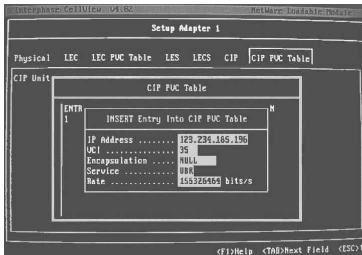
Figure 10-10. PVC Settings for CIP Clients
